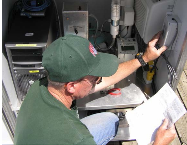
Ecology's Greg Hannahs calibrates automated monitoring equipment at the Walla Walla air monitoring site.
