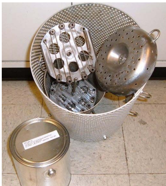
Figure 2. SPMDs Inside a 5-Membrane Canister and Inserted in a Shade Device Cylinder.
