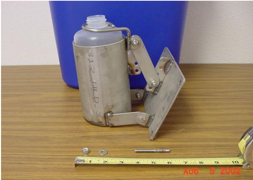
Figure 1. Modified Ecology Stormwater Sediment Bottle Trap. (Courtesy City of Tacoma)
