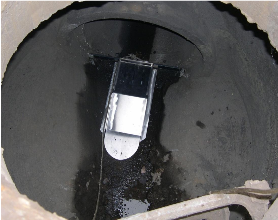
Figure 5. Example Deployment Configuration of the Hamlin Prototype Sampler.
