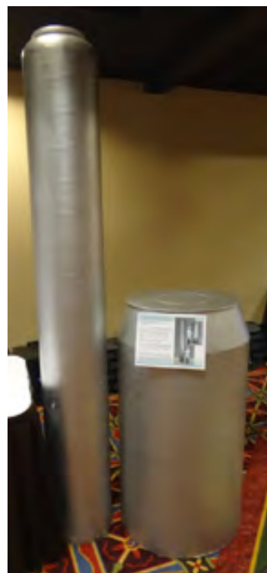
Left: Model ion exchange column (not to scale) that will channel cesium-137, a radioactive isotope, into the high-level waste stream for processing.
