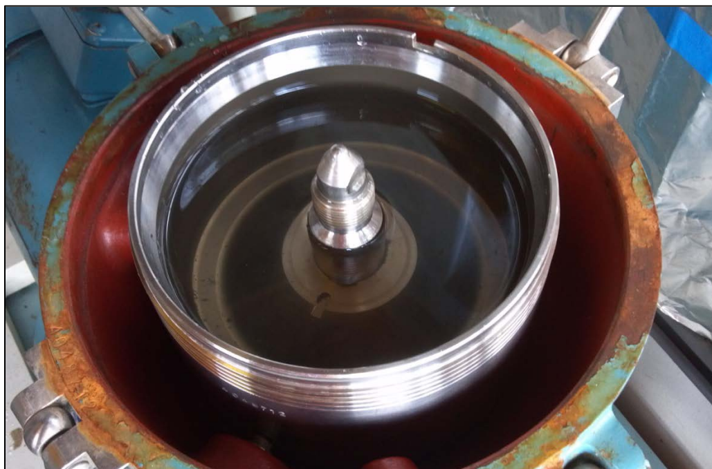
Figure 9. Centrifuge bowl with SSPM sample.
