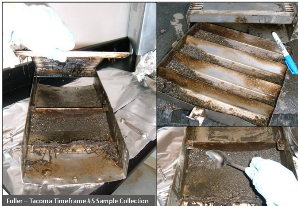
Figure 7. Fuller prototype sampler with SSPM sample.
