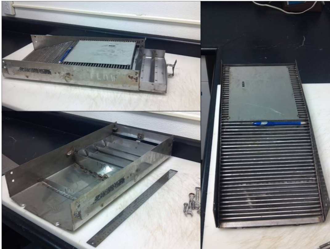
Figure 4. Fuller SSPM sampler Assembled (right), tray access (top left), and lower chamber with baffle and tray (bottom left).
