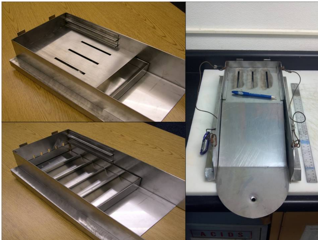
Figure 3. Hamlin SSPM sampler.
