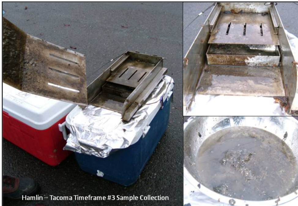
Figure 6. Hamlin prototype sampler with SSPM sample.
