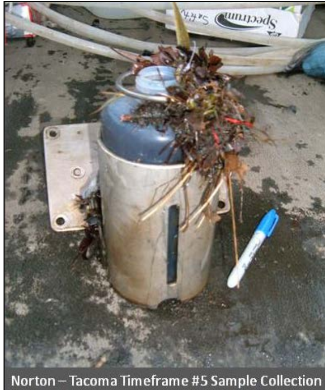
Figure 8. Norton bottle trap with SSPM sample.
