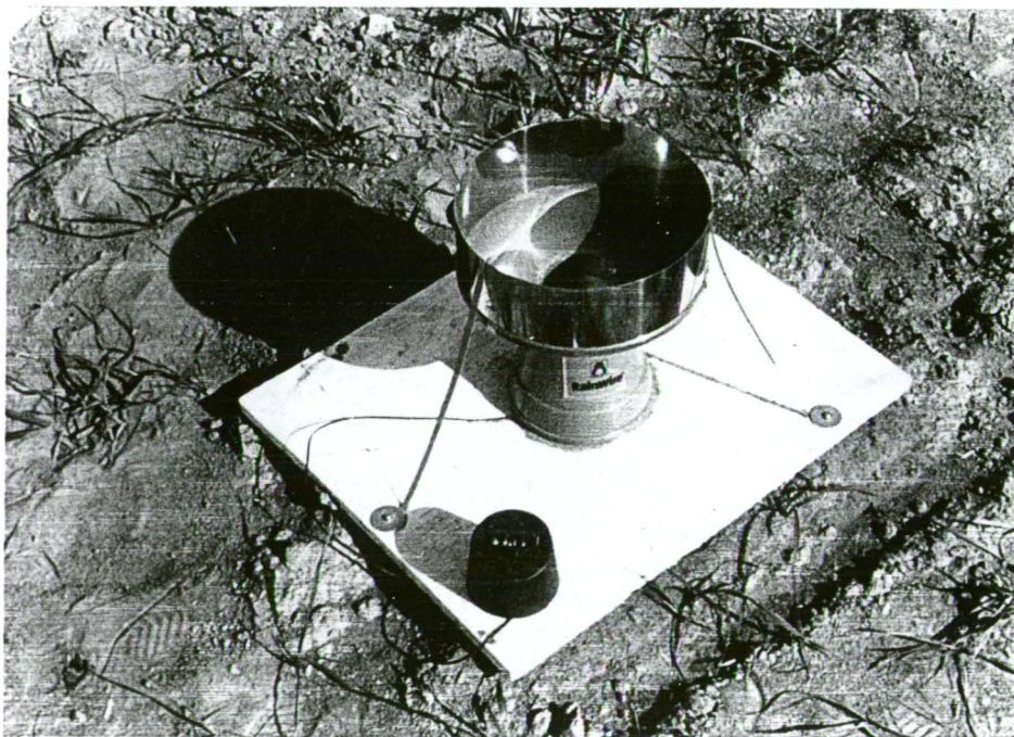
Recording precipitation gauge (catch pan and recorder).
