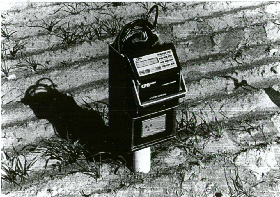
Neutron probe mounted on PVC access tube.
