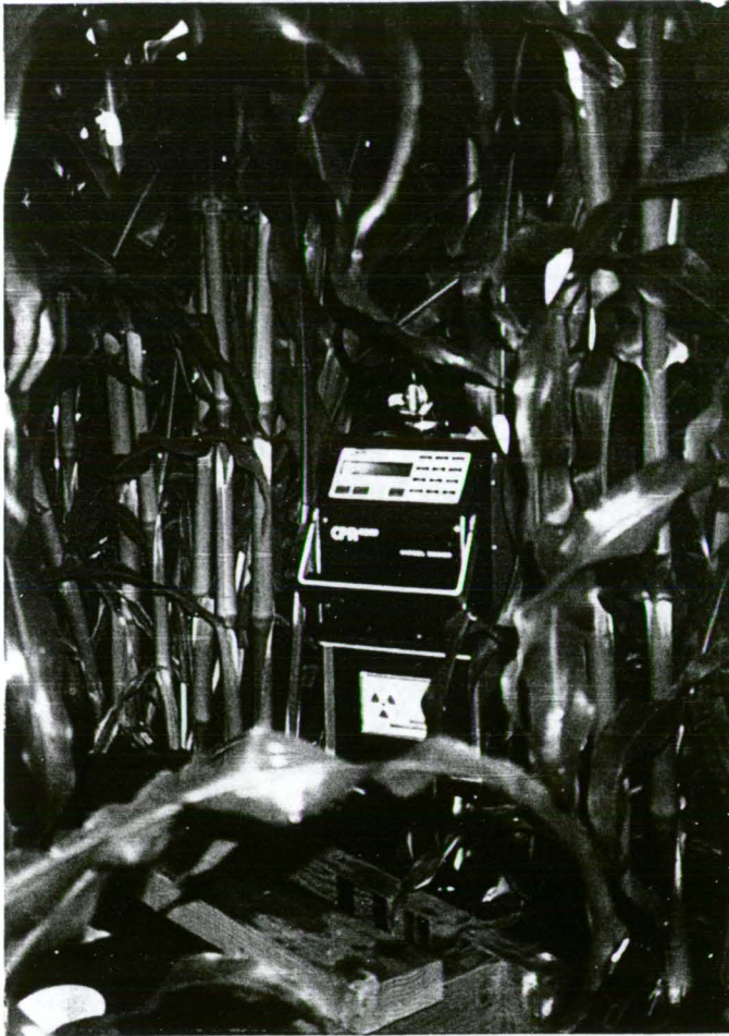
Neutron Probe on access tube in corn row. Note anti-compaction platform.
