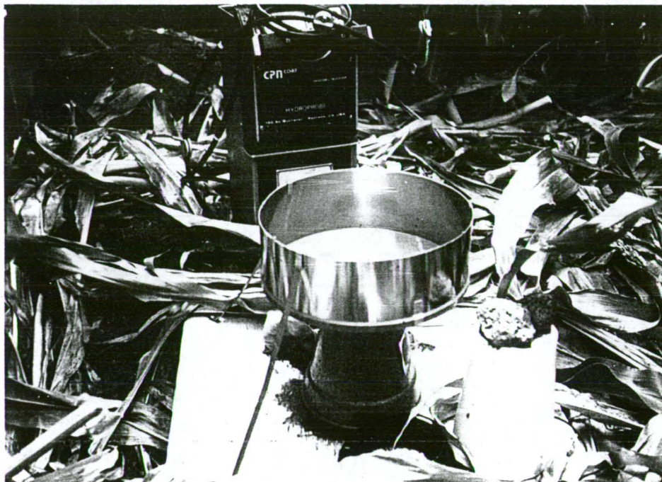
Recording precipitation gauge on site within crop clearing.
