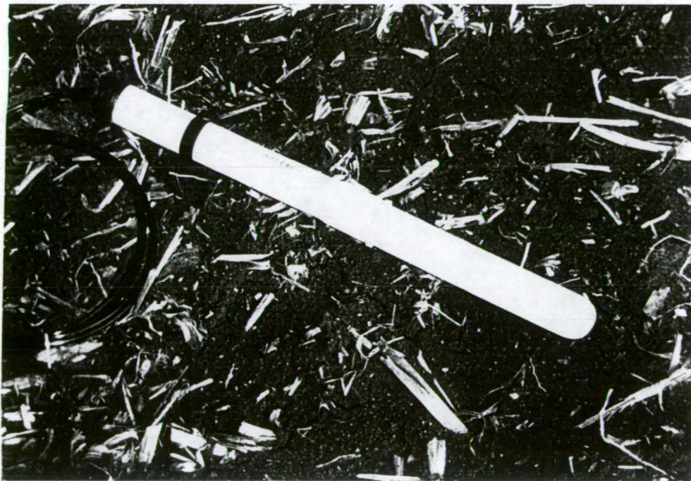
PLATE 7. BURIED VACUUM LYSIMETER WITH EXTENSION TUBING
