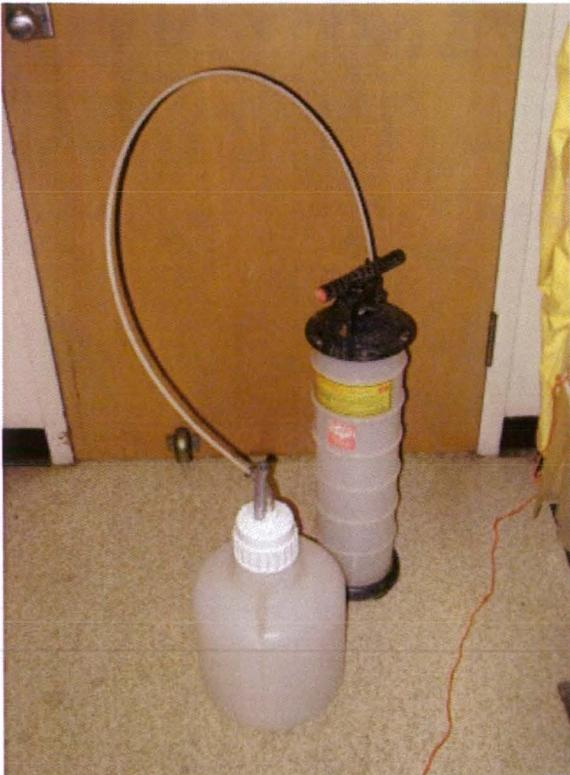
Figure 1. Vacuum pump connected to carboy.
