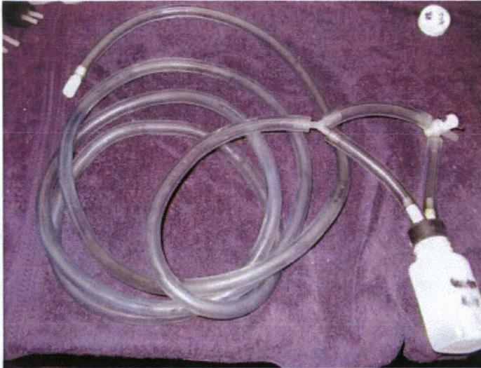
Figure 3. Collection tube with weighted Teflon tip is dropped into piezometer. Collection bottle and 3-way valve are described in Fig. 2.
