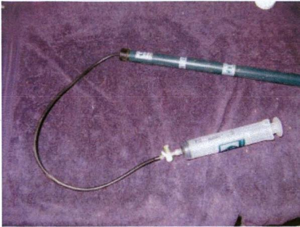
Figure 4. Soil solution sampler showing sampler, tubing, 3-way valve and syringe.
