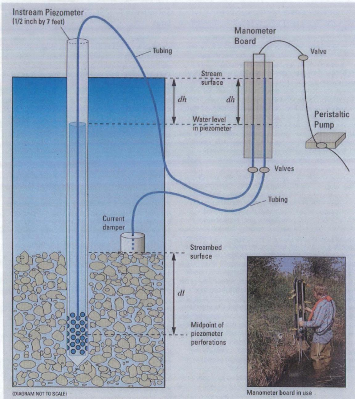
FIGURE 3-2\_ MANOMETER BOARD DIAGRAM
