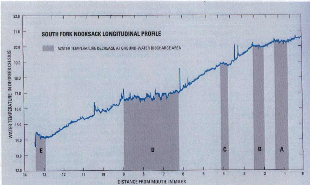
FIGURE 4-1 SOUTH FORK NOOKSACK RIVER LONGITUDINAL WATER TEMPERATURE PROFILE AT RIVER BOTTOM, FROM RIVER MILE 13.5 TO CONFLUENCE WITH NORTH FORK, AUGUST 28, 2003
