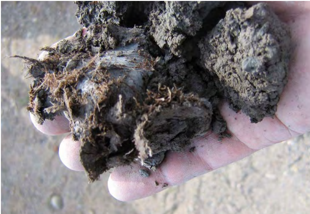
Photograph 2 – Organic Fibers at 116 feet bls
