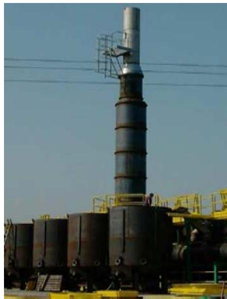
**Figure 8. Several batch pyrolysis reactors linked to an after burner known as a CML process (Source: [http://www.drveniugljen.hr/assets/files/prezentacije/06\\_Christian\\_Bedrossian.pdf](http://www.drveniugljen.hr/assets/files/prezentacije/06_Christian_Bedrossian.pdf)).**
