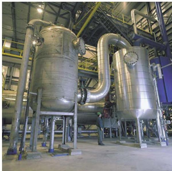
**Figure A4. A Pyrocycling™ system containing a two step condensation process**
