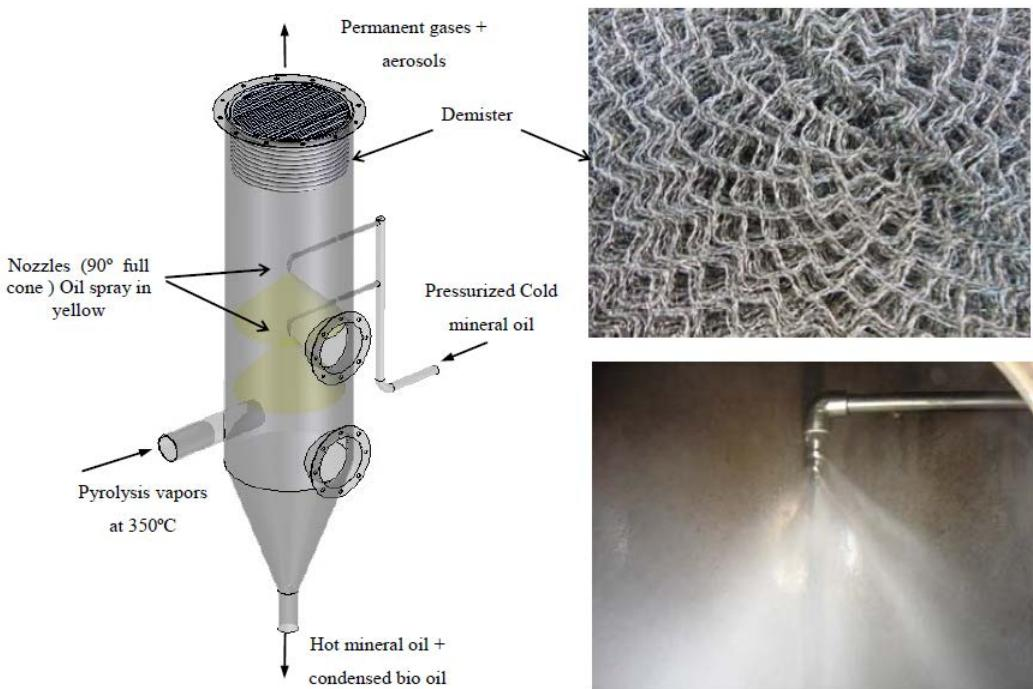
**Figure A6. Condenser of pyrolysis vapors (San Miguel et al. 2011).**
