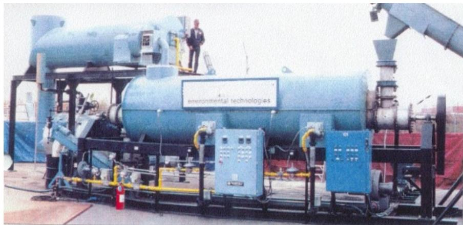
**Figure 9. The steam produced by this auger pyrolysis unit with a thermal oxidizer can be used to generate electricity. (Source: <http://www.internationaltechcorp.org/IT-info.htm#convert>).**
