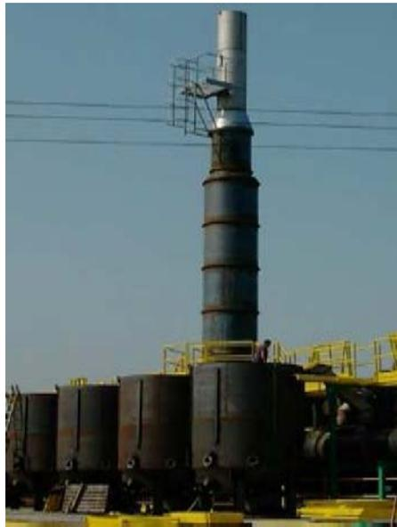
**Figure 8. Several batch pyrolysis reactors linked to an after burner known as a CML process (Source: [http://www.drveniugljen.hr/assets/files/prezentacije/06\\_Christian\\_Bedrossian.pdf](http://www.drveniugljen.hr/assets/files/prezentacije/06_Christian_Bedrossian.pdf)).**
