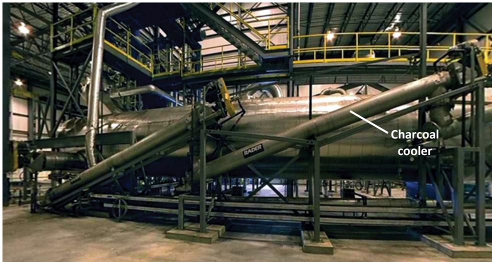
Figure 15. Charcoal cooling system in vacuum pyrolysis plant (Source: Group Pyrovac).
