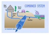
The CSO Project: The city recently bought a five-million gallon tank and 12.5 acres of property from Rayonier. The tank will hold excess stormwater and sewage during very heavy rains. This water will later be treated at the sewage treatment plant. To connect existing stormwater pipes to the tank, the city will install new pipes across the Rayonier property (see map on page 3).
