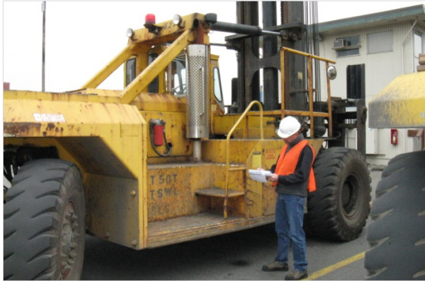
Frank Van Haren of Ecology's Air Quality Program inspects cargo handling equipment at the Port of Seattle to determine if the equipment is a suitable candidate for an exhaust emission control device.
