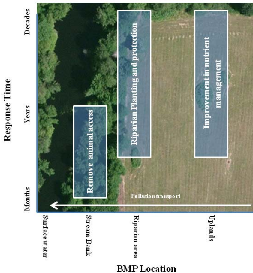
Figure 3. The scale of common BMPs and their typical response times. Modified from Mesner, 2011.
