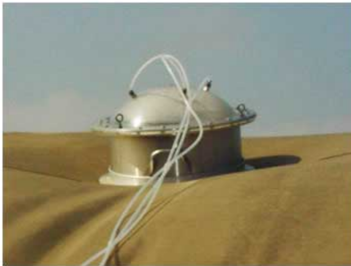
Figure 1 - Flux chamber emission sampler
