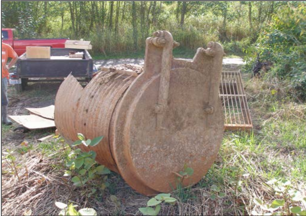
Old 48-inch flapper valve tide gate
