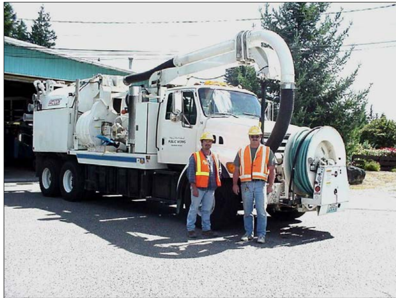
Figure 31. Vactor Truck used to clean out stormwater catch basins.
