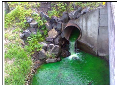
Dye testing to determine illicit connection of a sanitary sewer to a stormwater outfall Photo credit: Pullman Stormwater Services
