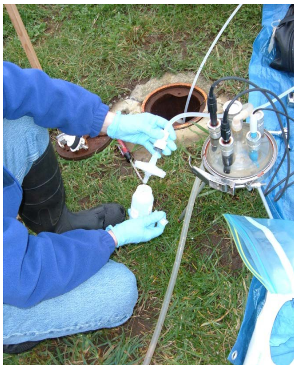
Figure 15. Field-filtering a groundwater sample using a disposable, in-line filter that bypassed the flow cell.
