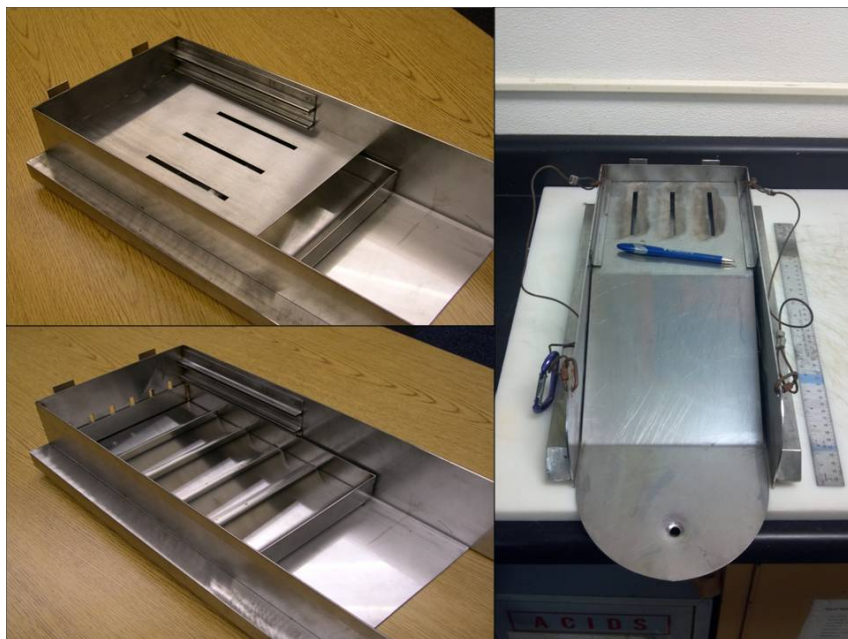
Figure C-1. Hamlin sediment trap for collection of suspended sediments.
