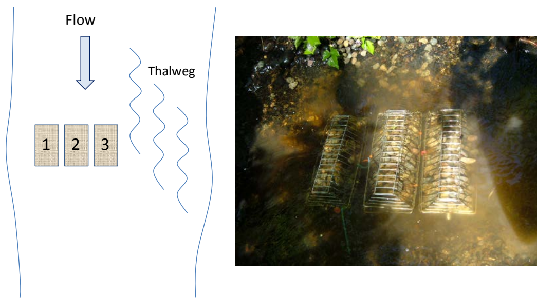
Figure 5. Diagram (left) and photo (right) of hatchbox in-substrate deployment method.
