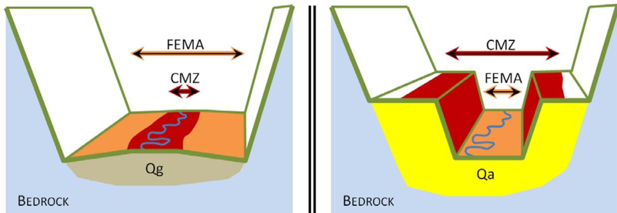
**Figure 8. CMZs versus FEMA floodplains.** Schematic illustrations of valleys where the FEMA floodplain (orange) is wider than the CMZ (left), and the CMZ (red) is larger than the FEMA floodplain (right). The stream in the left panel is underfit, as indicated by the Quaternary glacial outwash (Qg) composing the valley floor. The stream on the right has incised (cut into) a deposit of Quaternary alluvium (Qa) susceptible to lateral channel erosion.
