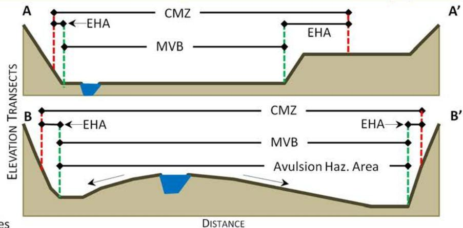
**Figure 5. Schematic diagram of a pCMZ. Schematic elevation profiles (A→A' and B→B') are shown to illustrate relative elevations of valley bottom features and their relationship to pCMZ map units. In cross section B → B', note the cross-valley gradients and the associated indications of avulsion hazard. Mapping of the CMZ shown is discussed in detail throughout the text.**
