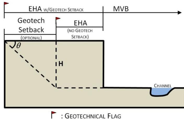
**Figure 7. Cross-sectional illustration of geotechnical hazards and pCMZ map units. The pCMZ designations are shown for scenarios in which the optional Geotechnical Setback is and is not mapped. The required Geotechnical Flag is shown mapped in both scenarios. The Geotechnical Setback distance depends on landform height (H) and assumed failure angle ( $\theta$ ). Figure modified from Rapp and Abbe (2003).**
