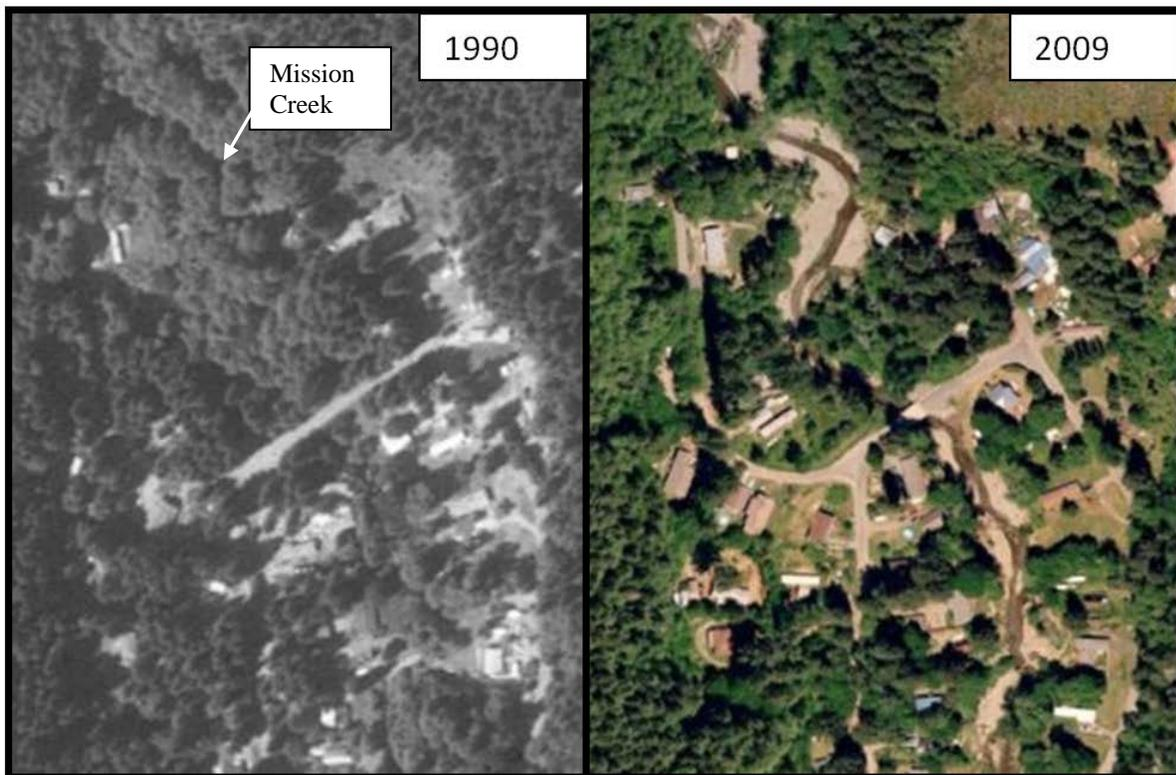
**Figure 3. Example of channel widening. Mission Creek near Belfair, WA illustrates channel widening between 1990 and 2009, and its encroachment on the adjacent community.**
