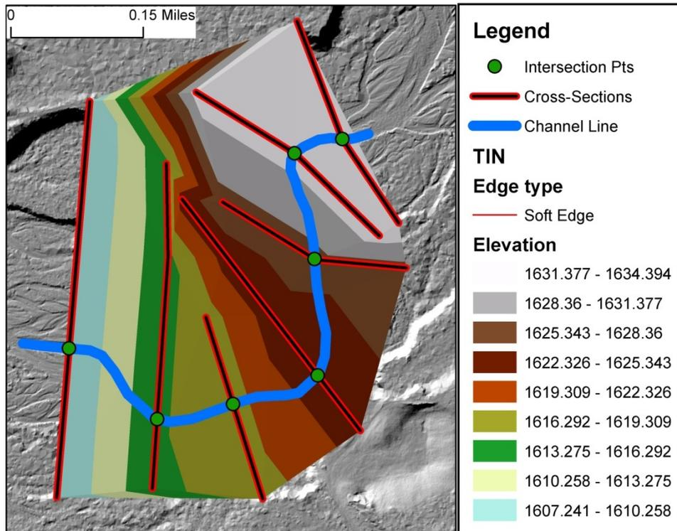
**Figure 8:** Map of TIN created using the cross-sections shown.
