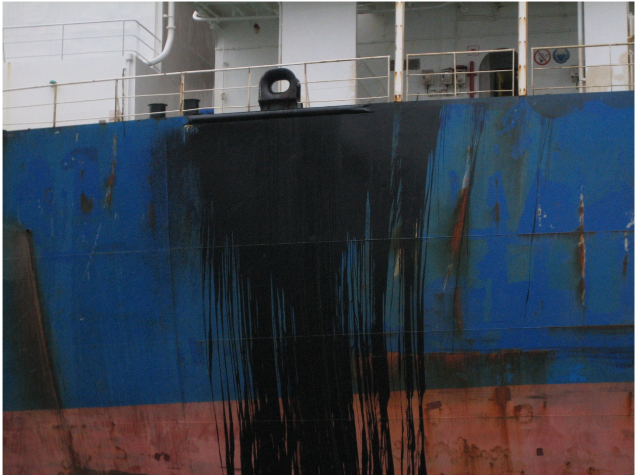
Figure 3 - Result of inattention during a bunkering operation at anchor.
