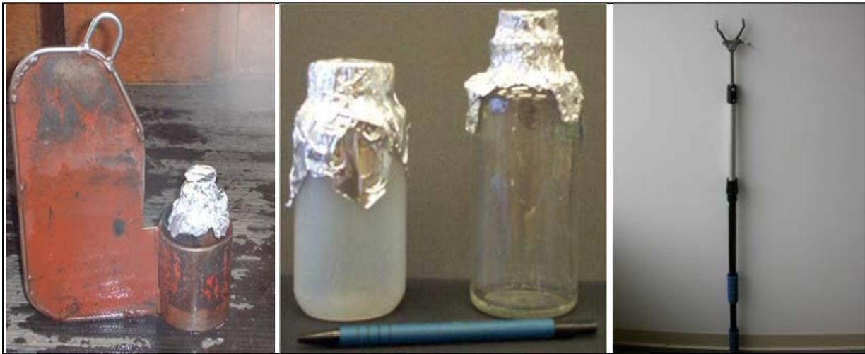
**Figure 1. Bacteria water sampling equipment and sample bottles.** *Left: Specialized bridge sampler with bottle. Center: 250 mL polypropylene and glass sample bottles. Right: Sampling extension pole.*
