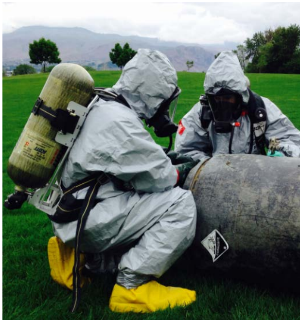
Anna Harris and Jim Pearson, after-hour spill responders from the Central Regional Office, sample an abandoned drum for hazard characterization and safe disposal in Wenatchee.
