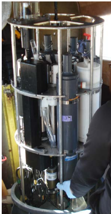
Figure 4. Sea-Bird Electronics, Inc., Conductivity, Temperature, Depth (CTD) instruments and other sensors in a custom-made frame.
