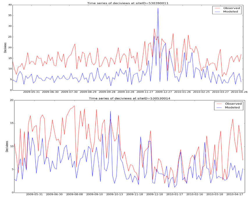
Figure C.16: Comparison of modeled and observed deciviews at Wishram (top), and Mt. Rainier (bottom)
