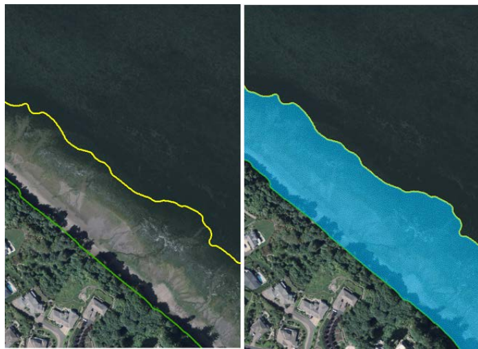
Figure 6: (Left) Both MHHW and MLLW tidal datum line could be generated from single CZMIL LiDAR dataset. (Right) Foreshore features consist of the area between MHHW and MLLW. Topobathymetric LiDAR and VDatum provide an easy and consistent method of extracting tidal datum lines.
