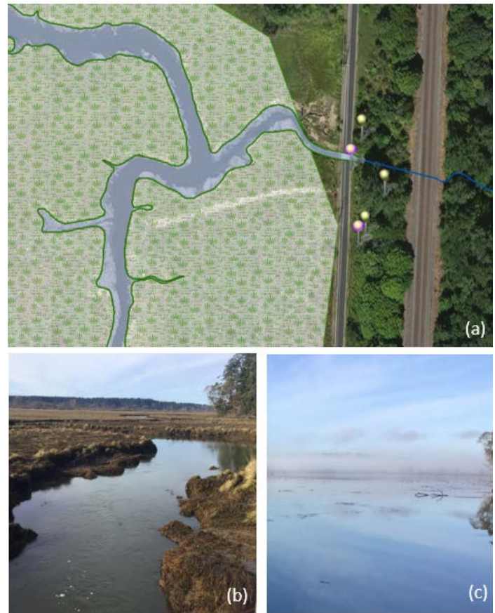
Figure 5: (a) Screenshot from Esri’s Collector app shows added points of interest and swamp/marsh feature collected while in field. (b) Channels at MHHW line, correspond to LiDAR-derived shoreline. (c) Same location but at king tide (2.03 ft higher than MHHW on 1-14-16).
