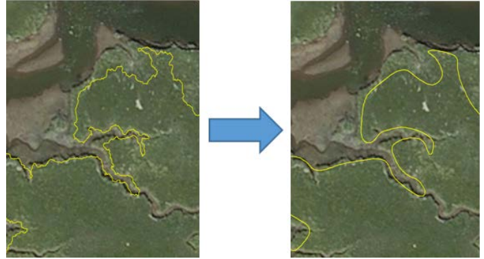
Figure 3: (Left) Original MHHW contour from LiDAR. (Right) MHHW shoreline after being generalized and smoothed using ArcMap's generalization toolset. (Images at 1:600 scale)
