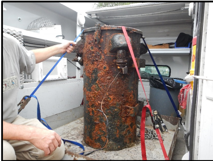
Figure 18: Removal of intact transformer from the Wenatchee River near Aplets Way Bridge in Cashmere.
