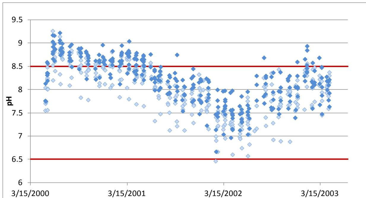
Figure 2. Time-series plot of all pH measurements made by the Okanogan CD for the grant project (#G0000225) in comparison to pH criteria of 6.5 to 8.5.
