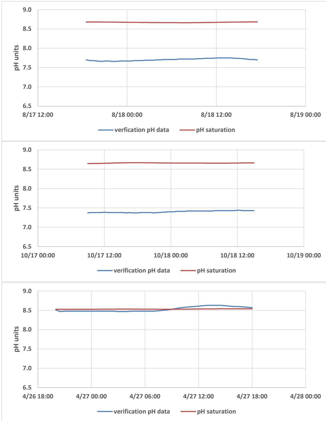
Figure 12. Results of pH time series for Siwash Creek verification monitoring in August and October 2015 and April 2016.
