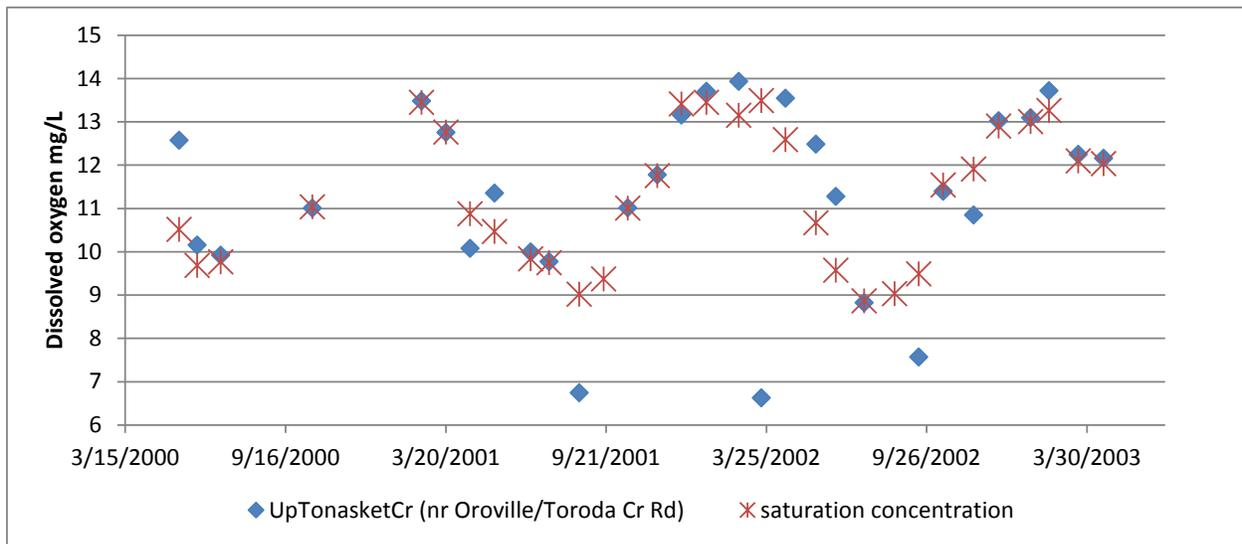
Figure F-9. Okanogan CD dissolved oxygen data compared to saturated levels for upper Tonasket Creek.
