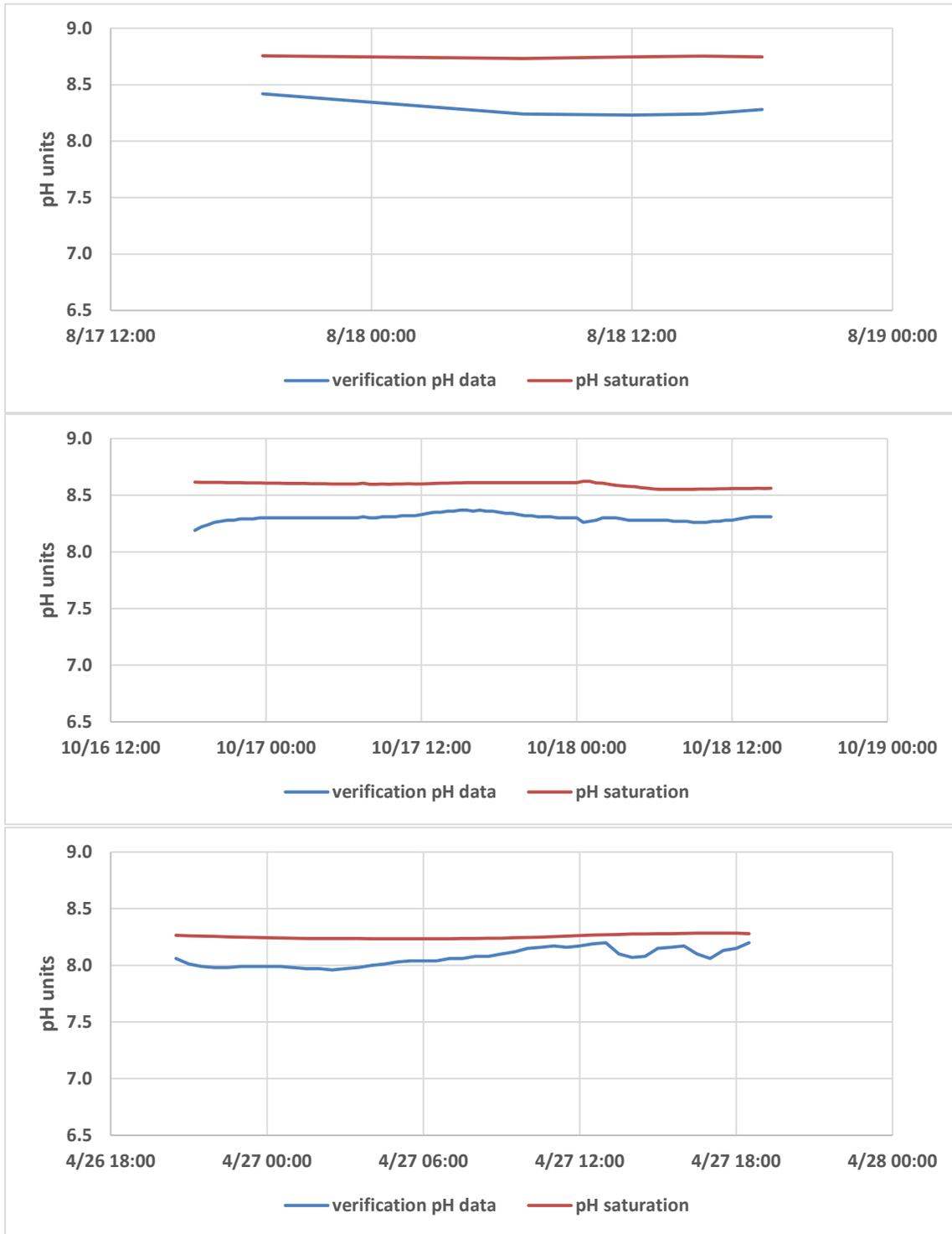
Figure D-3. Results of pH time series for Bonaparte Creek verification monitoring in August and October 2015 and April 2016 compared to the pH saturation.
