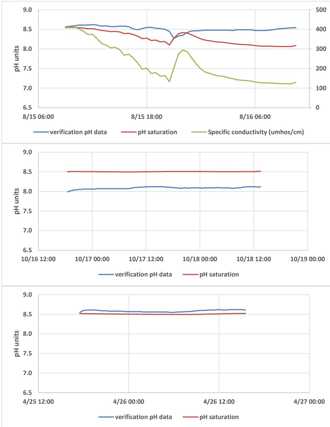
Figure 15. Results of pH time series for Chiliwist Creek verification monitoring in August and October 2015 and April 2016.
