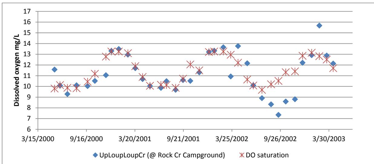
Figure F-10. Okanogan CD dissolved oxygen data compared to saturated levels for upper Loup Loup Creek.
