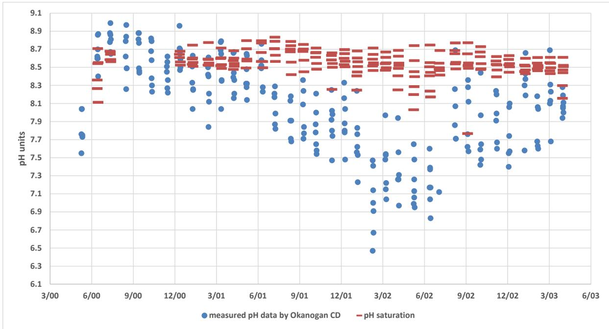
Figure 4. Comparison of measured pH data by the Okanogan CD in three tributaries and the calculated pH saturation in the same tributaries.
