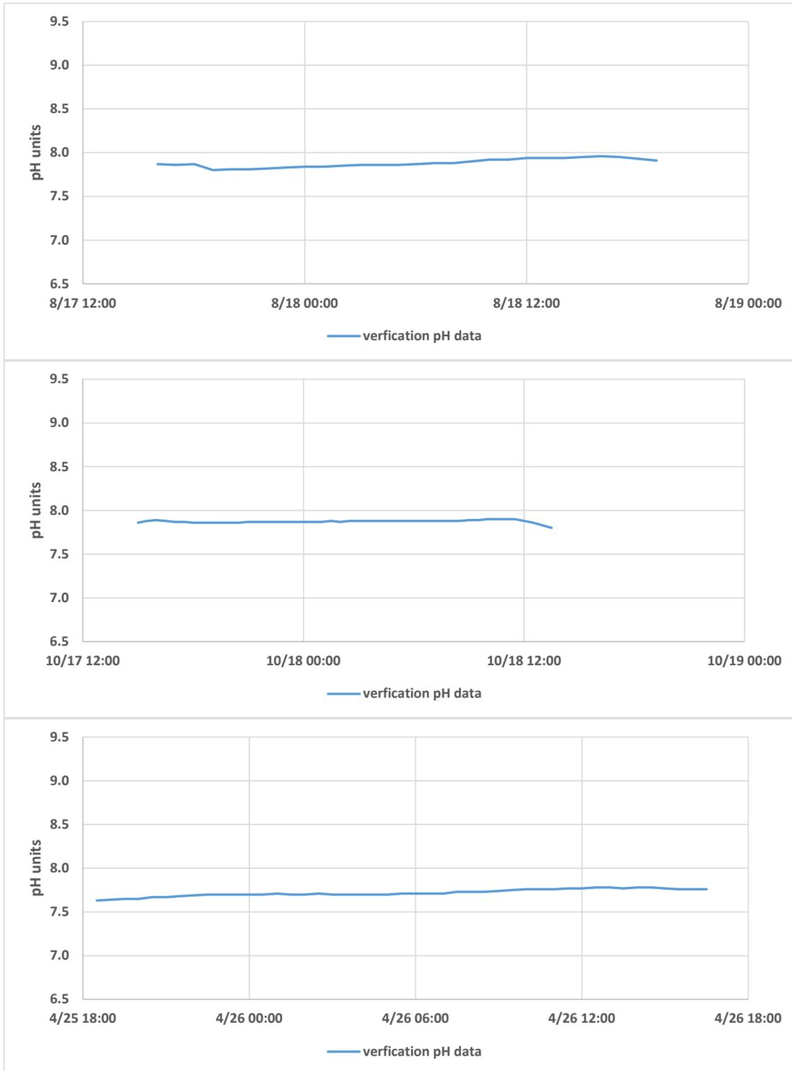
Figure 9. Results of pH time series for Tallant Creek verification monitoring in August and October 2015 and April 2016.
