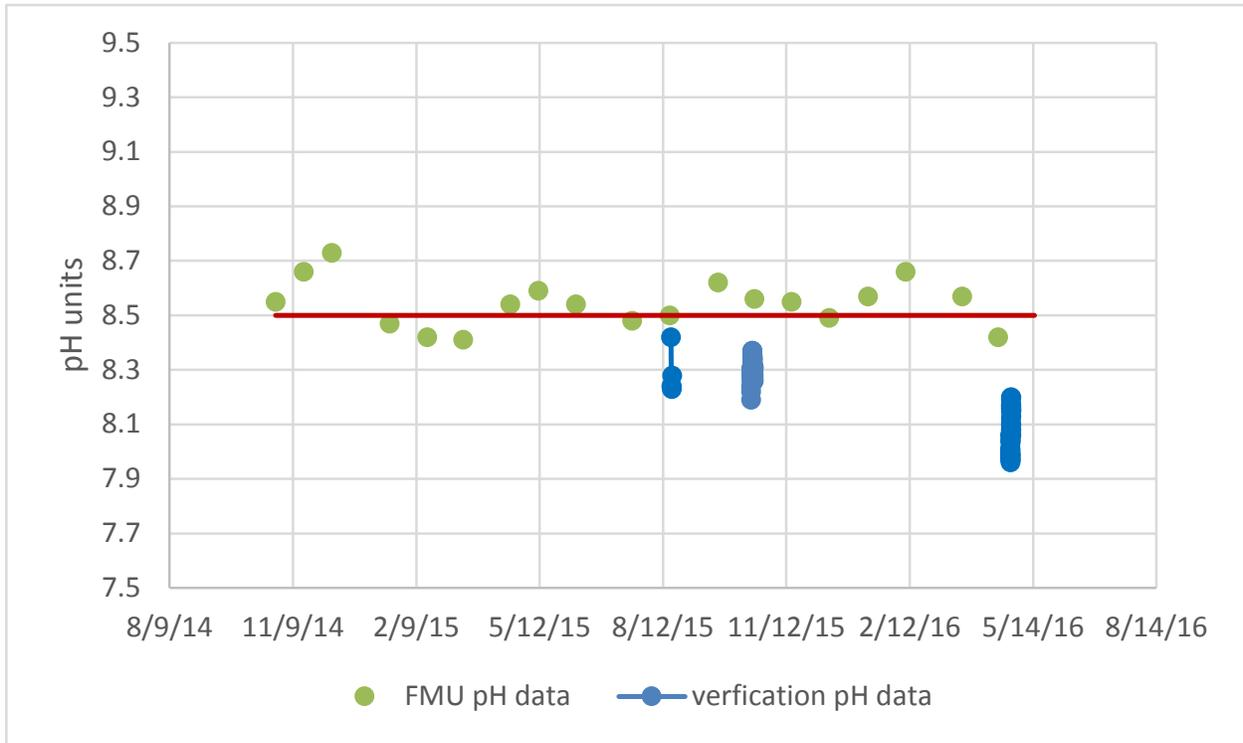
Figure D-1. A comparison of FMU pH monitoring of Bonaparte Creek to the continuous in situ pH monitoring from the verification study.
