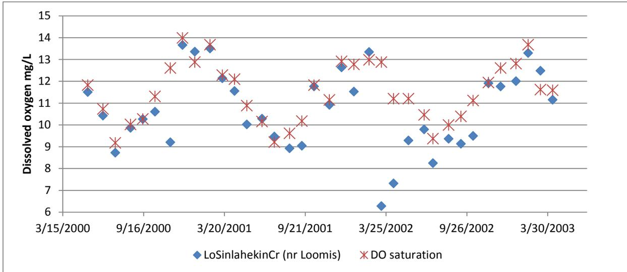
Figure F-1. Okanogan CD dissolved oxygen data compared to saturated levels for lower Sinlahekin Creek.
