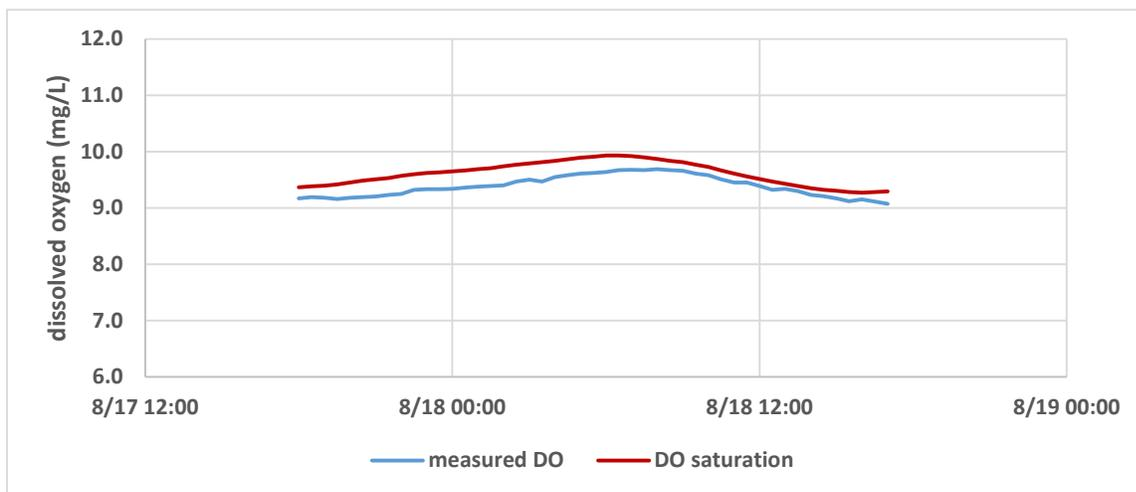
Figure F-6. Verification study dissolved oxygen data compared to saturated levels for lower Ninemile Creek in August 2015.
