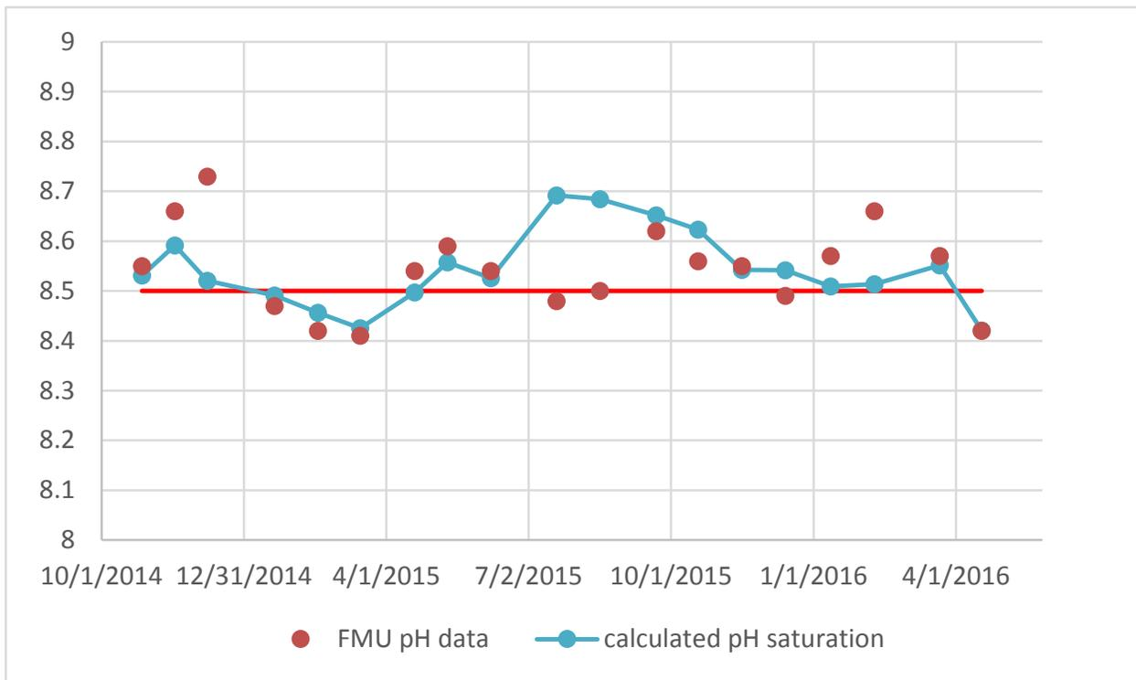
Figure D-2. A comparison of FMU pH monitoring of Bonaparte Creek to calculated pH saturation.
