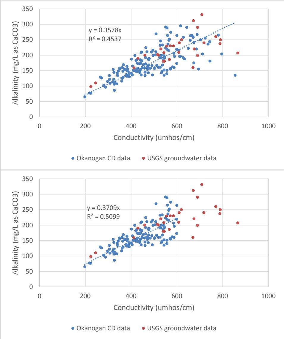
Figure C-2. Regression between conductivity and alkalinity using Okanogan CD surface water data and showing relationship to USGS groundwater data for the Okanogan basin.
