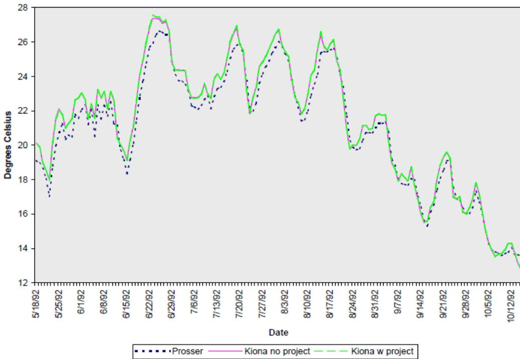
Figure 8. Simulated mean daily water temperatures with Project (green) and without Project (magenta), upstream and downstream of the Chandler Powerhouse under 1992 conditions. Water temperatures at Prosser Dam (blue) were measured in 1992.
