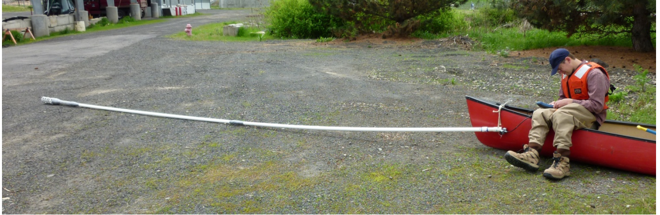
Figure 1. PVC assembly for carrying Hydrolab MiniSonde® along streambed behind small watercraft.
