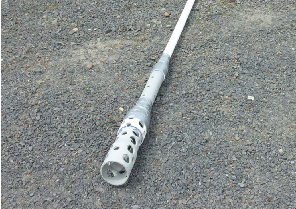
Figure 2. Hydrolab MiniSonde® properly seated inside PVC cage.
