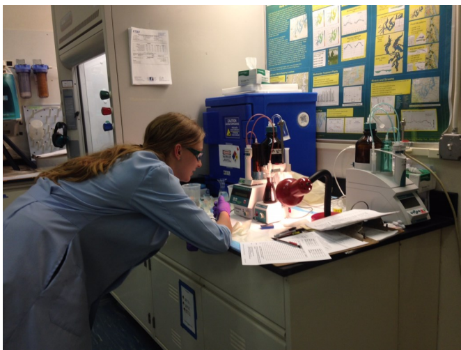
Analyzing seawater samples collected on a sea plane flight in Puget Sound for dissolved oxygen using the Winkler Method.
