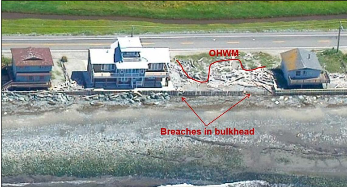
Figure 4-23: Breach in bulkhead resulting in relocation of OHWM.
