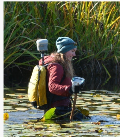
Hannah collecting elevation data on foot with GPS backpack on and GPS controller in hand. Photo submitted by Hannah Drummond.
