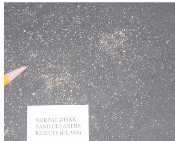
Photo 2. Glass in the Paper Bales – Sample Rejected by Sand Cleaner Source: NORPAC 2009
