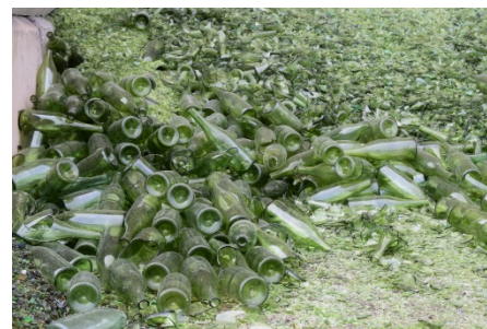
Photo 5: Container glass becomes cullet (broken or whole scrap glass) which manufactures back into glass containers. Photo courtesy of Recology CleanScapes.
