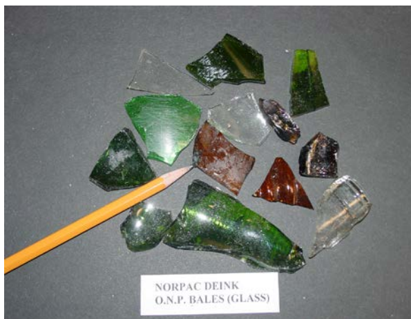
Photo 1. Glass in the Paper Bales – Sample Rejected after Drum-Pulper Pulping Process Source: NORPAC 2009
