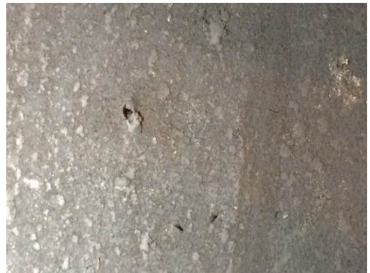
Photo 7: Damage to a conveyor belt at a MRF due to glass. Glass shards moving through the system can cause punctures and tears, causing belts to wear out more quickly than they would if glass were not in the stream. Photo courtesy of Recology CleanScapes.
