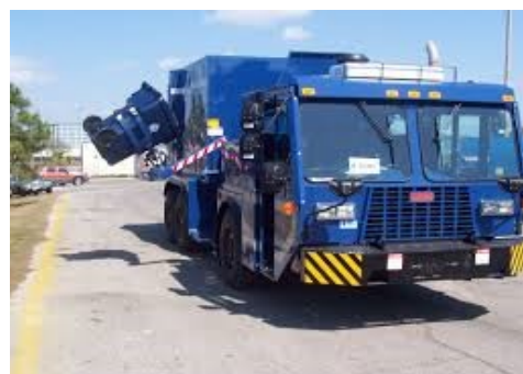
Photo 2: Recycling truck with automated arm for lifting the commingled recycling cart.
