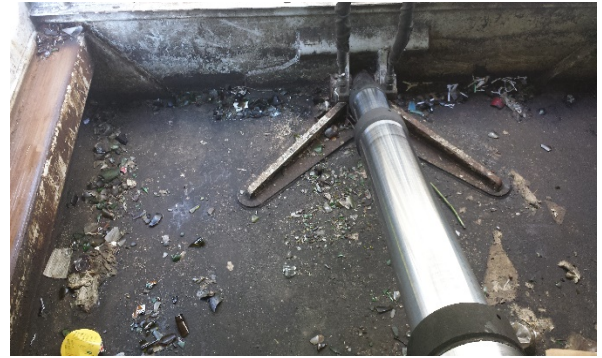
Photo 6: Glass is abrasive on truck compaction floors.
