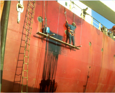
Side of ship being cleaned after a fuel oil overflow involving failure of a tank level gauging system and overflow alarm.
