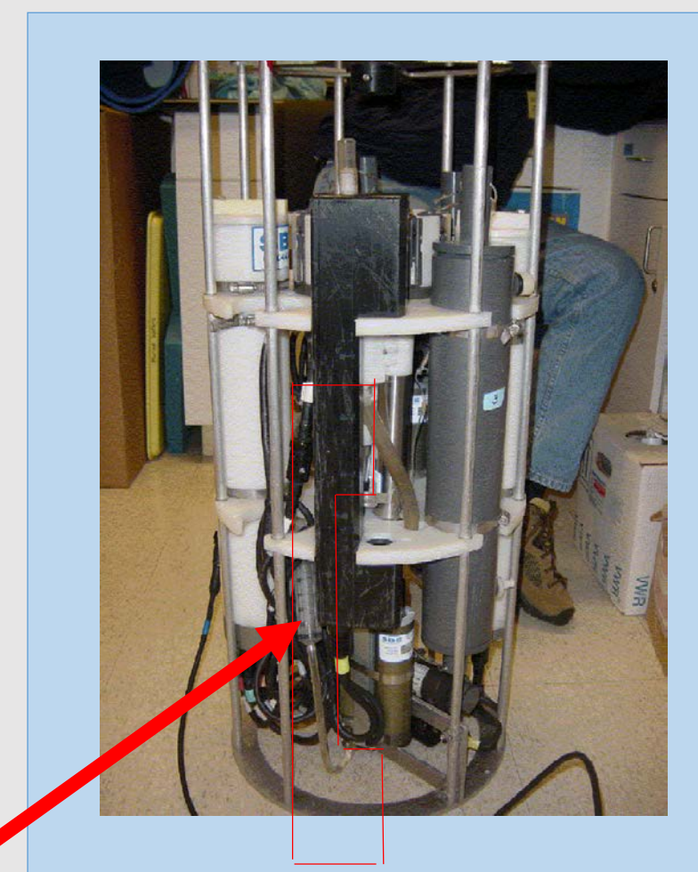
Figure 1. CTD package with arrow locating the light transmissometer.
