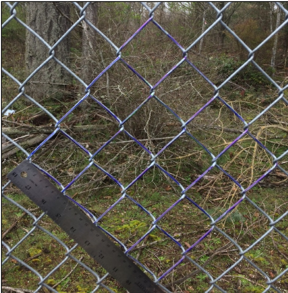
Figure F-2. Chain-link fence test area (2-inch mesh spacing).
