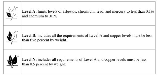
Figure 1. Package Markings Indicating Level of Compliance of Brake Friction Materials
