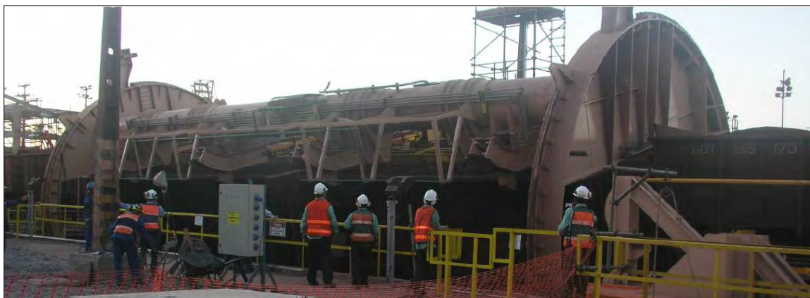
Figure 2-5. Typical Tandem Rotary Unloader
