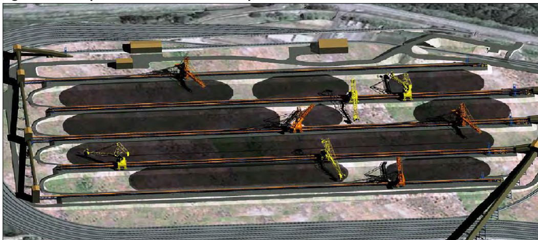
Figure 2-6. Representation of the Stockpile Area with Stackers and Reclaimers
