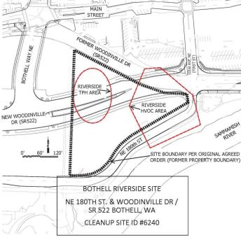
Several interim cleanup actions have occurred throughout the Bothell Riverside Site. In 2010 and 2017, two separate soil excavation and removal actions were conducted to address the petroleum impacts at the Riverside TPH area.
