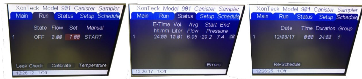
Figure 3: Run (left), Status (middle), and Schedule (right) menus on the front panel control
