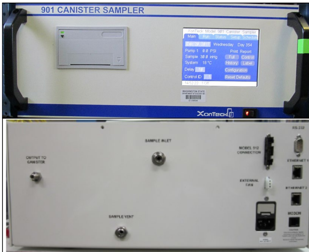
Figure 2: Xontech 901 Canister Sampler front panel (top) and rear panel (bottom)
