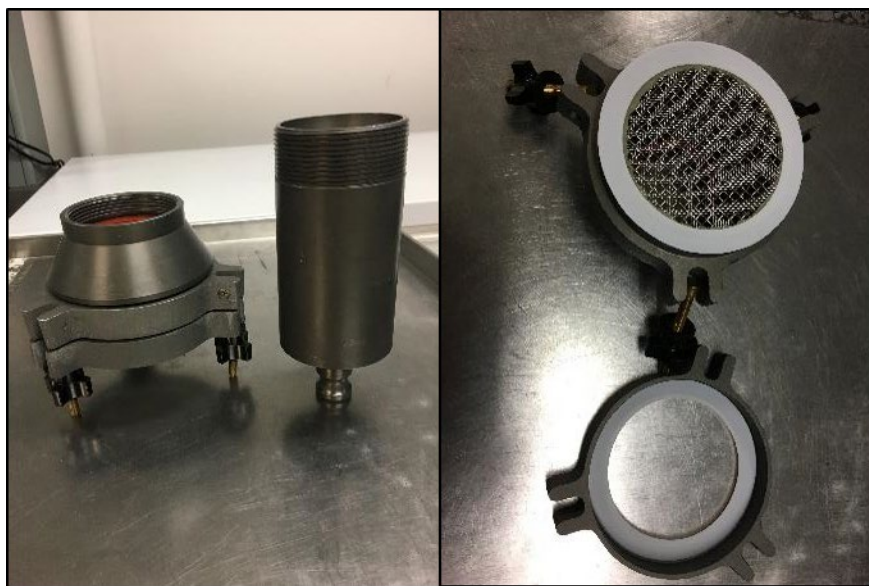
Figure 10: Separated dual chamber sampling head (left) and particulate filter holder (right).
