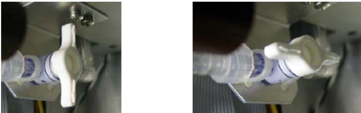
Figure 8: Purge valve closed (Left) and open (Right). Located inside the battery compartment
