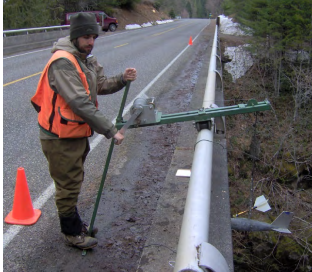
Figure 1. Bridge board equipped with a USGS Type A reel. (Photo by Washington Dept. of Ecology)
