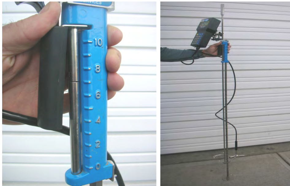
Figure 10. Wading rod with meter set at six tenths of a depth of 1.7 feet. (Photo by Washington Dept. of Ecology)
