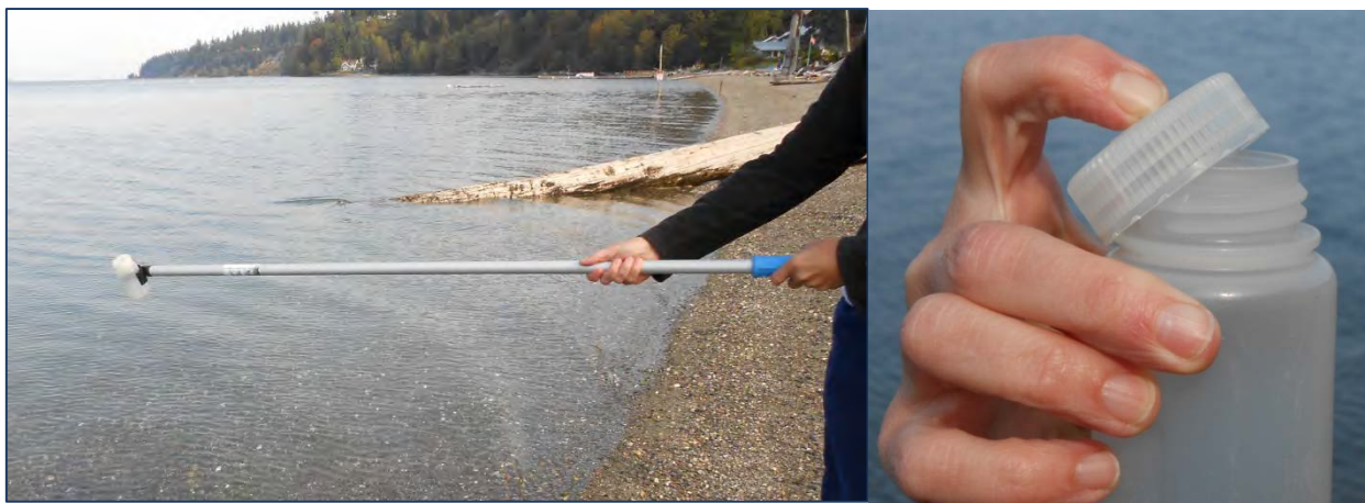
Figure 1. Left: Sampling extension pole with bottle. Right: Bottle with small opening between bottle and cap.
