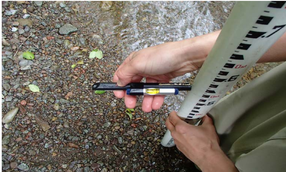
Figure 5. Measuring bankfull height using a surveyor's rod and laser level.
