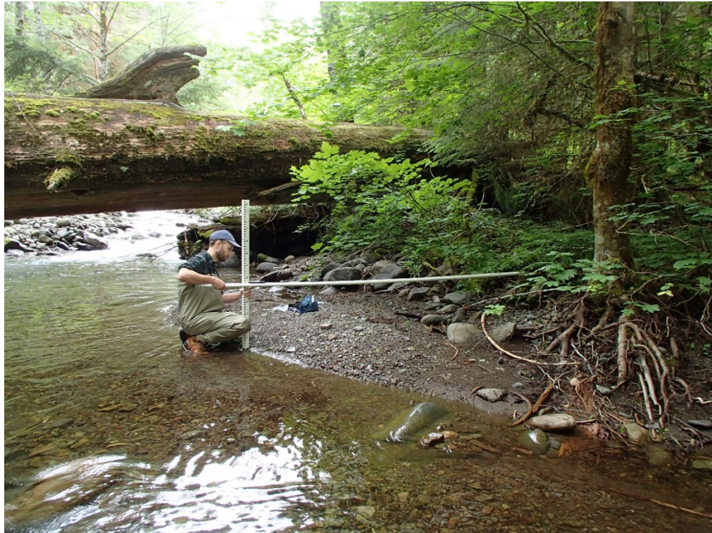
Figure 6. Measuring bankfull height using a surveyor's rod and hand bubble level.
