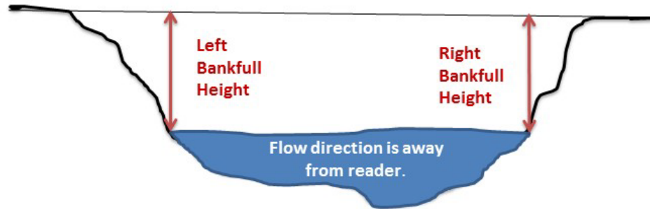
Figure 4. Diagram of the left and right bankfull height measurements.
