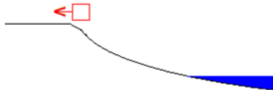
Figure 4. Densiometer station at one bank of each major transect for the Wide Protocol . Bank choice is determined by Table 1 of Hartman (2017).
