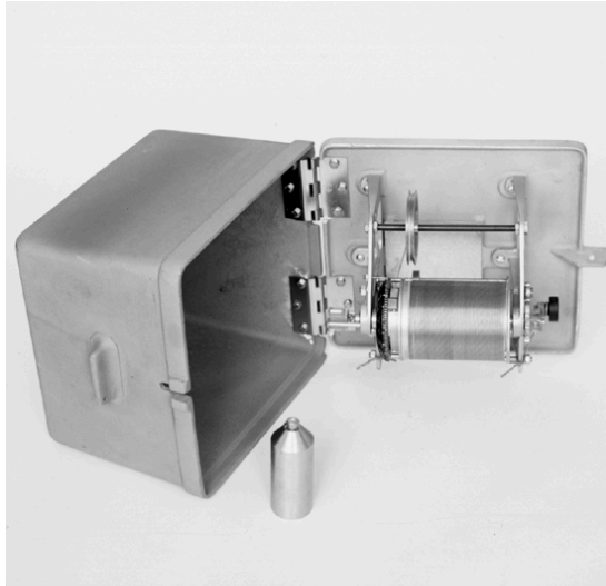
Figure 2. Wire Weight Gage (photo courtesy Rickly Hydrological Company)
