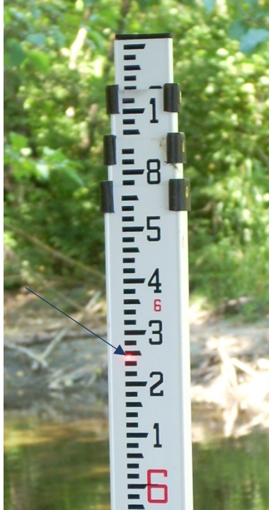
Figure 7. The center of the bright red laser light dot projected on the rod is the point at which the stadia rod is read. (Photo by Washington Dept. of Ecology)
