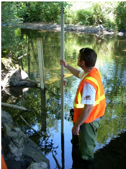
Figure 8. Hold the rod perpendicular on solid substrate in calm water. (Photo by Washington Dept. of Ecology)
