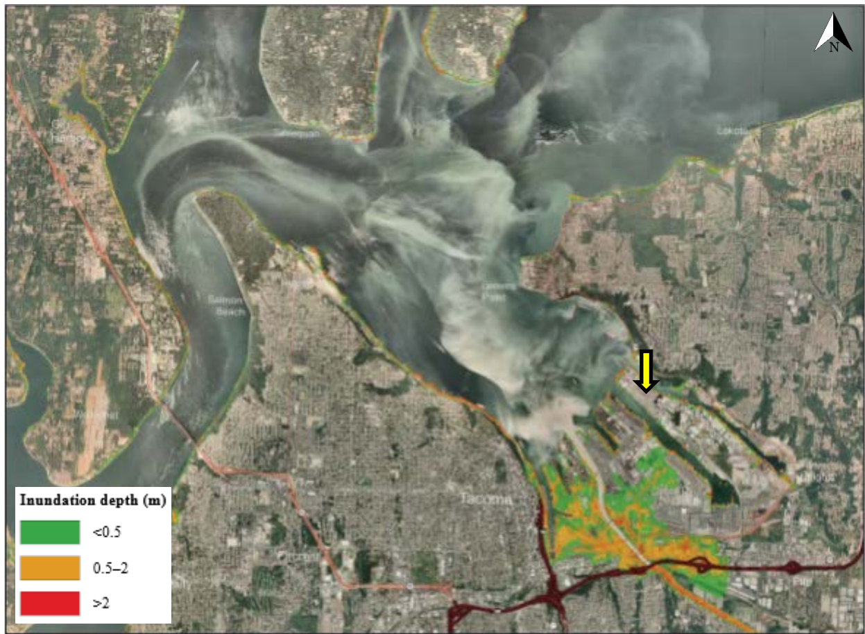
Figure 5: Modeled inundation from a tsunami induced by a magnitude 7.3 Tacoma-Rosedale Fault earthquake (Walsh et al., 2009). A yellow arrow indicates the approximate location of the Occidental Site. 1:62,500 map scale.
