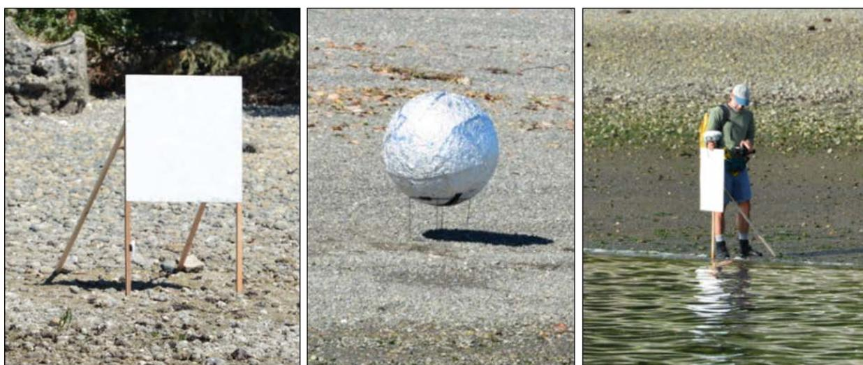
**Figure 8: Lidar ground-control targets; left—rectangular sheet metal, middle—spherical, right—surveyor measuring the location of a target**
