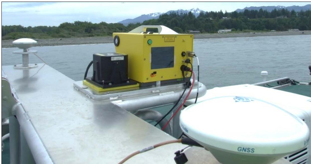
**Figure 5: Laser scanner and IMU mounted to the cabin top of the R/V *George Davidson***
