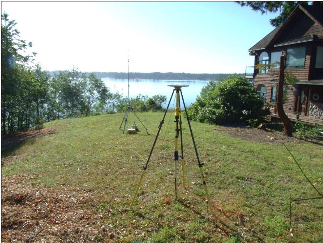
**Figure 6: Local RTK-GNSS base station set up at survey site**
