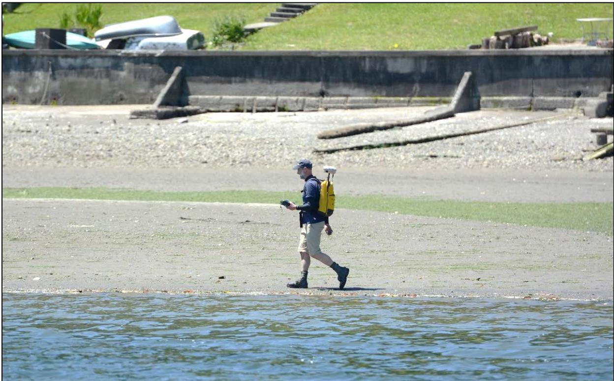
**Figure 7: Surveyor collecting RTK-GNSS beach topography data**
