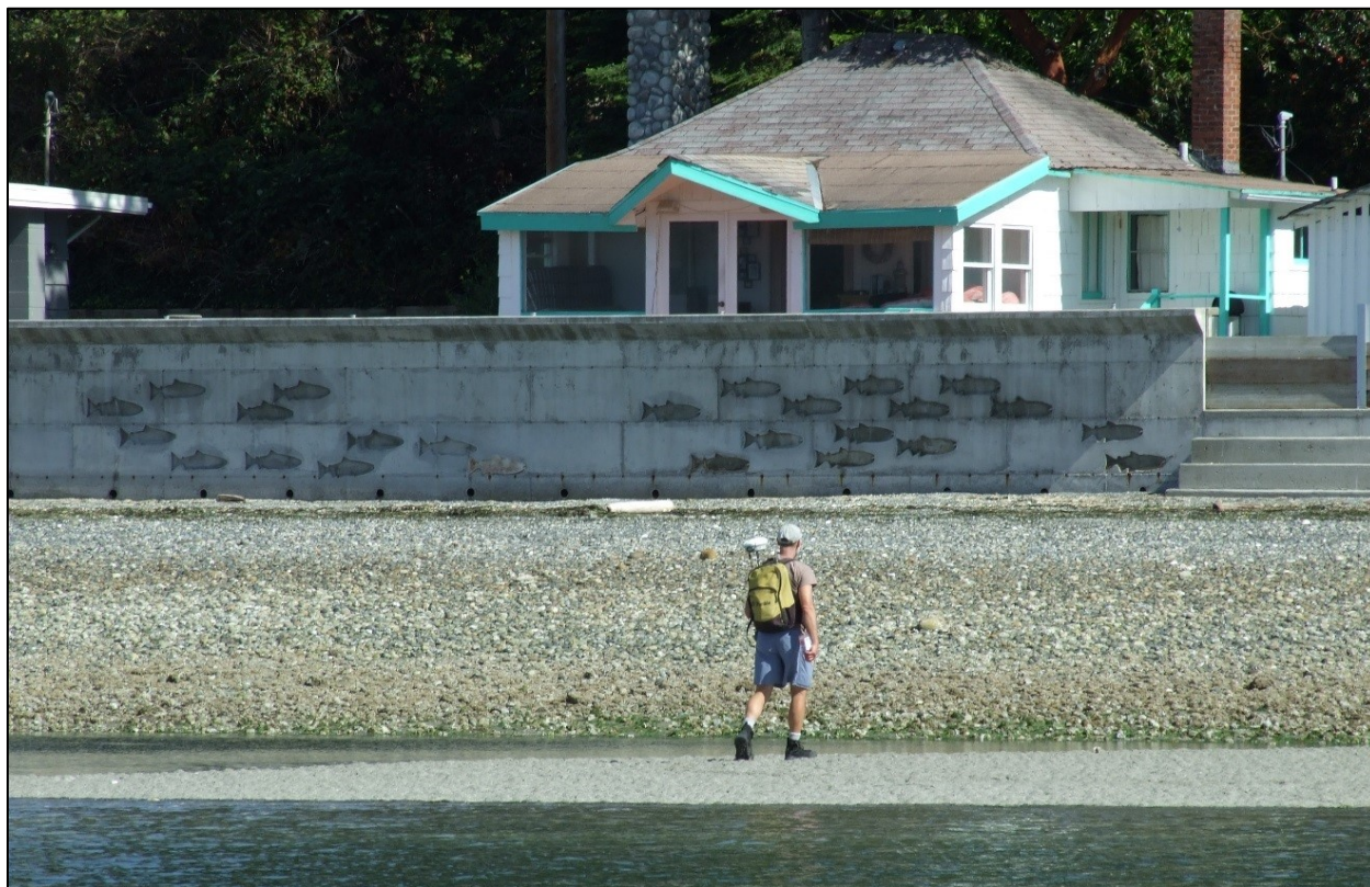
Figure 10: Photo of surveyor collecting beach topography data using a GNSS receiver mounted to a backpack
