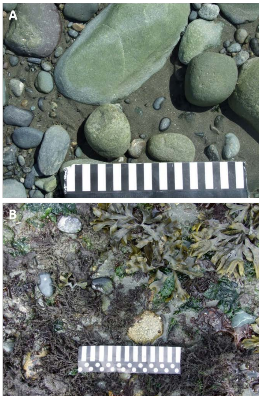
Figure A-3: Example beach types that present challenges when using automated tools to process sediment grain size photographs; (A) occurrence of large cobbles and sand together results in bimodal grain size distribution, (B) excessive organic matter covering surficial sediments makes it difficult to distinguish individual grains
