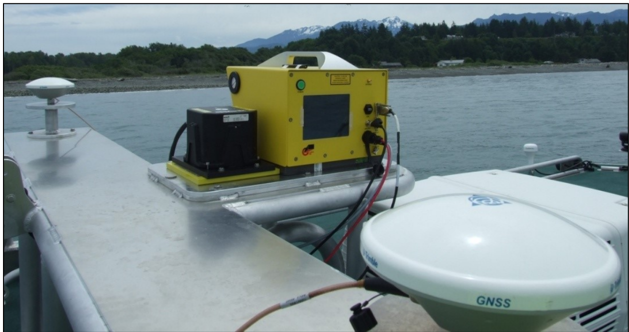
Figure 7: Photo of equipment used for mobile lidar surveys (Optech ILRIS-HD-ER laser scanner and POS MV V5 320 RTK system) mounted to a cabin-top platform
