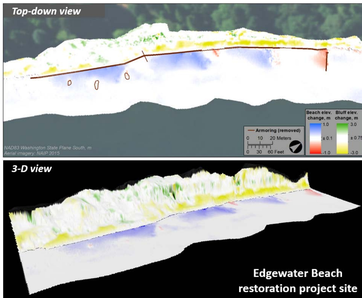
Figure E-34: 3D beach and bluff elevation change measured using boat-based lidar between September 2015 and June 2017 at Edgewater Beach [excerpted from Weiner and Kaminsky (2018)]
