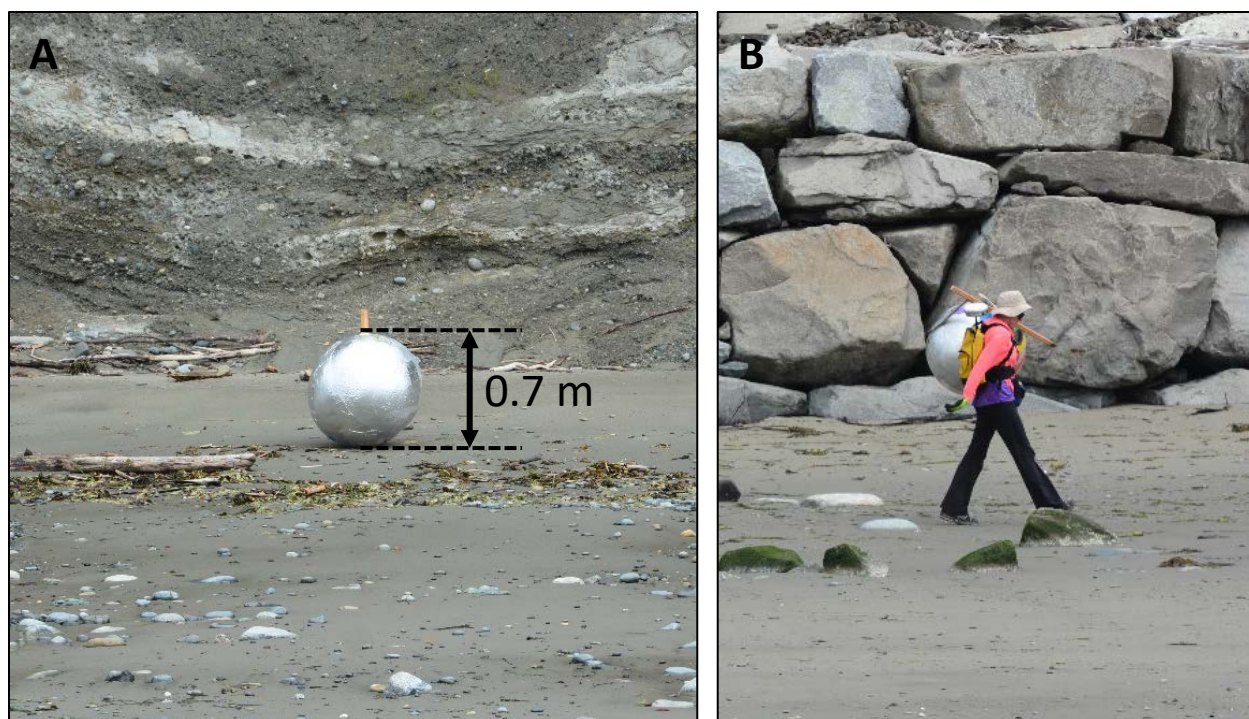
Figure A-2: Photos of prototype spherical ground control target: (A) target set up on the beach during the Ledgewood survey; (B) ground-based surveyor carrying target to another location
