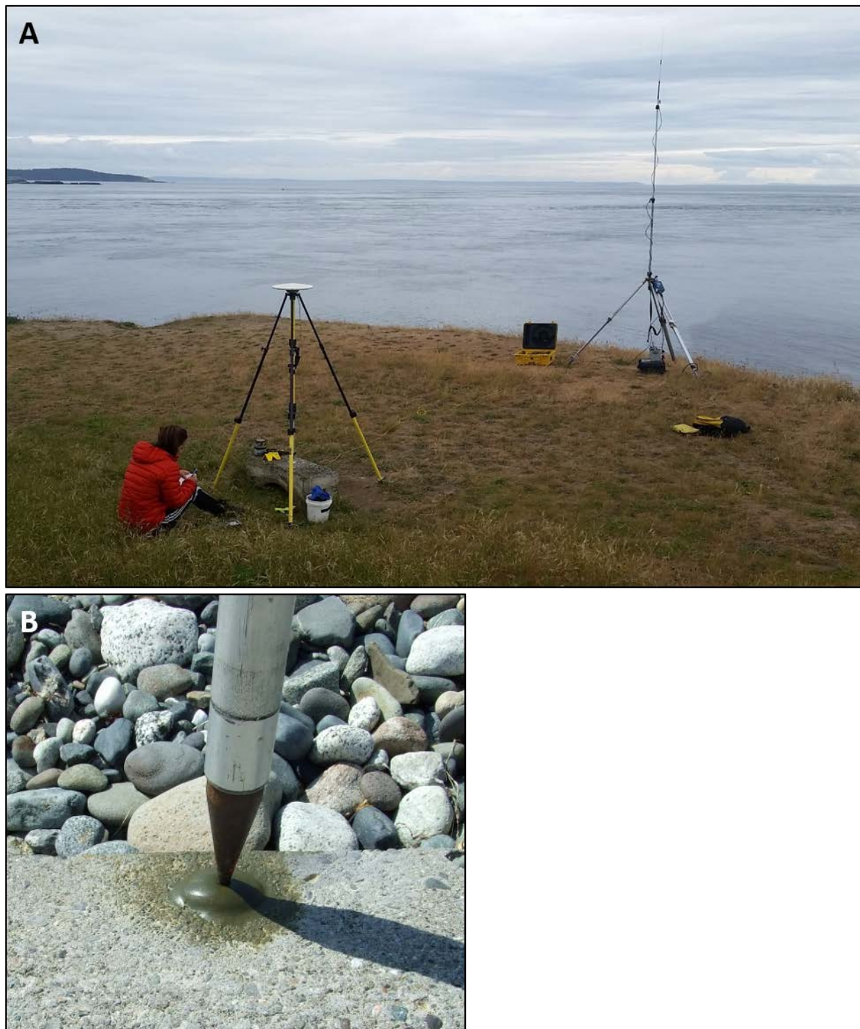
Figure 6: Photos of GPS base station setup: (A) GPS and radio tripods used for RTK surveying at Cattle Point; (B) epoxy monument installed on concrete slab for base station setup during Marrowstone Island surveys
