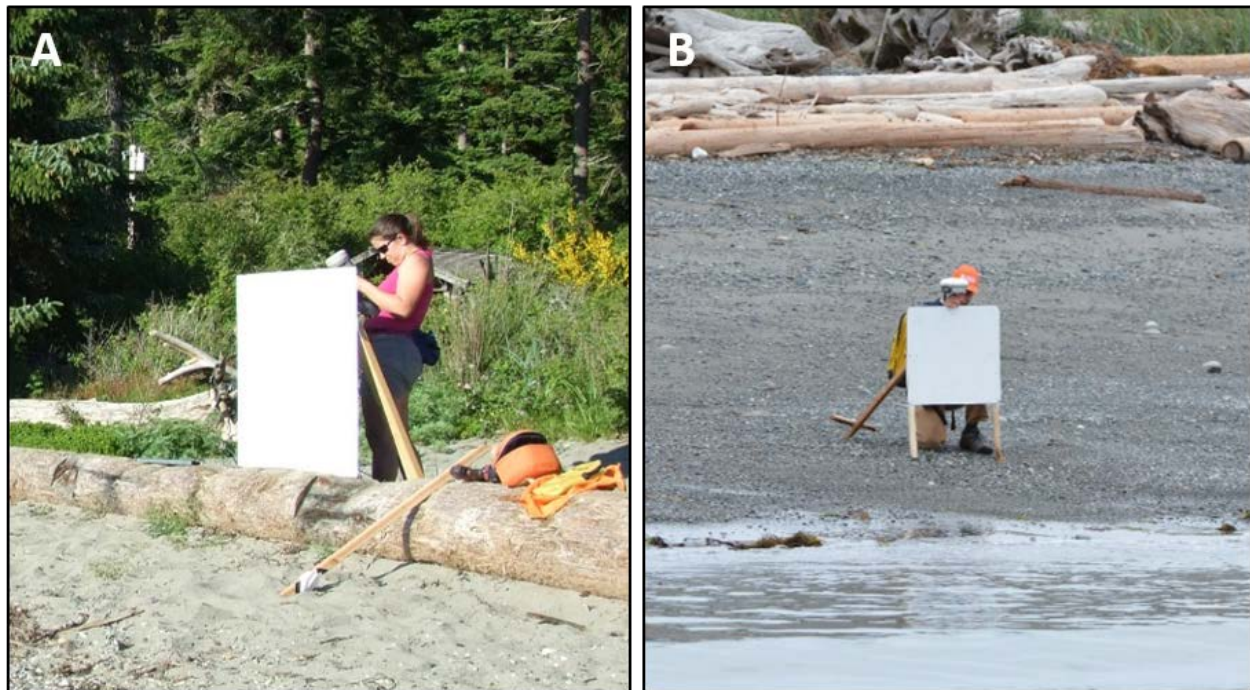
Figure 9: Photos of ground control targets used during boat-based lidar survey: (A) 1 m 2 sheet metal, spray-painted flat white; (B) smaller, light-weight sheet metal (0.77 x 0.61 m)
